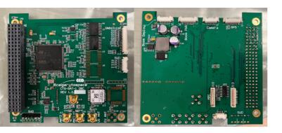
CalgaryToSpace has successfully designed, assembled and qualified the onboard computer that will run all satellite operations.
